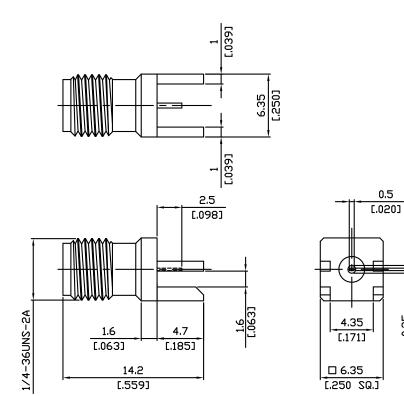
All dimensions are in mm [inch] Tolerances according to DIN ISO 2768-mH
